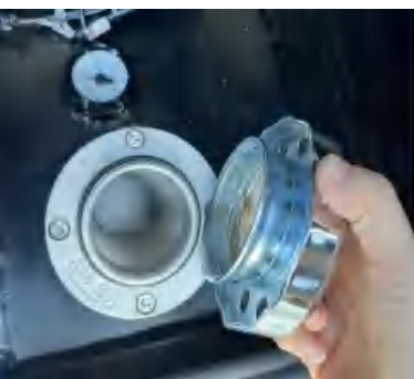
Stainless fuel filler tested at -45 degrees
