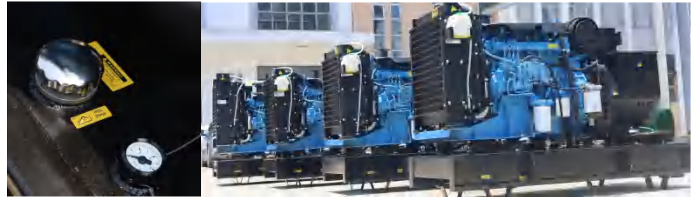
Protection function Test: ①Low fuel level alarm ②Low oil pressure alarm ③ High coolant temp alarm ④ Low coolant level alarm
